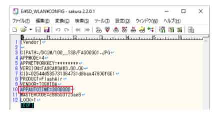
With the above work, the setting is completed. Please copy and paste all files / folders under SD\_WLAN in the downloaded ZIP file into the SD\_WLAN folder, remove it, and plug it into the SD card shield.
