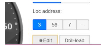
When you press the button, you can operate the locomotive at that address.
