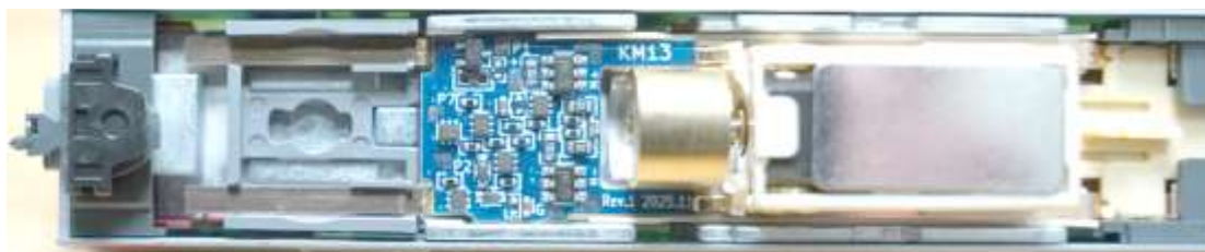
Example of installing KM13 in a friendly vehicle
