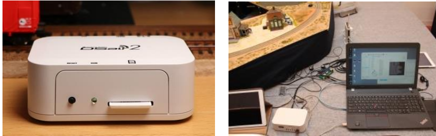
DSair2 and DSmain Arduino based DCC/MM2 digital command station system ( https://desktopstation.net/wiki/doku.php/dsair2_ukeng )
