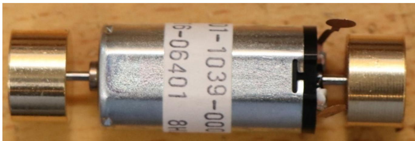
Solder wires and motor pins. Then set motor and floor parts.
